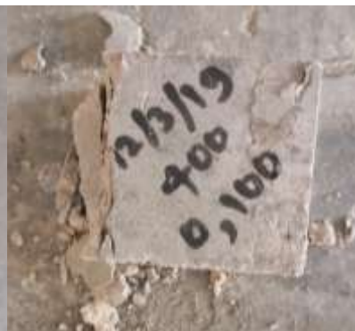
Fig.17: Test samples of GPM 200, GPM 400 and GPM 600 cubes
