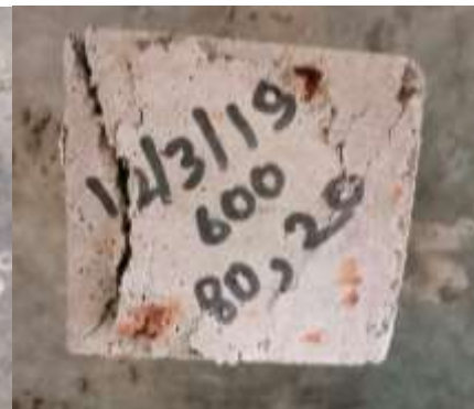
Fig.17: Test samples of GPM 200, GPM 400 and GPM 600 cubes
