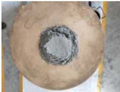
Fig 14: Flow table result 2
